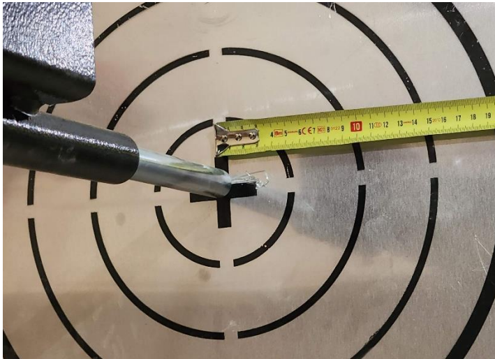
Scratch plate indicating approx. 4 cm maximum movement
