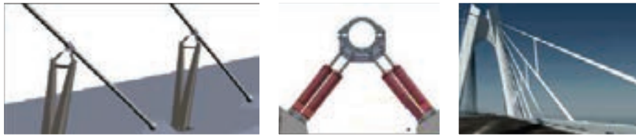
Figure 20. Viscous dampers and the cross-links used on the Yavuz Sultan Selim Bridge stay cables
